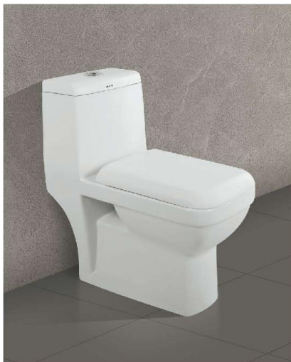
702 - ONE PIECE TOILET L 700 W 360 H 720mm Roughing In 'S' 230mm, 'P' 100mm
